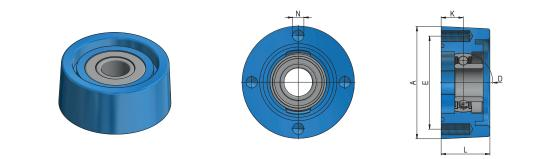
Circular Cast Housing Unit with Bearing - LSGR type Designation of Housing Unit with Bearing Dimensions mm 1111 D Е L Κ Α Ν 99 52 82 43 19,5 4xM10 LSGR205FS
